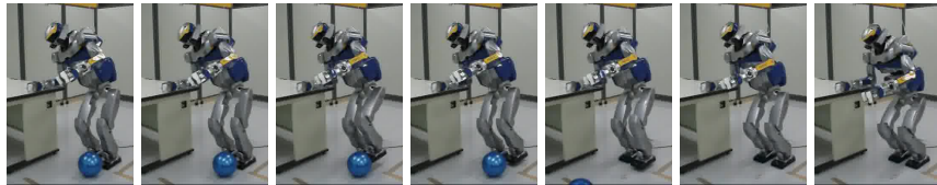
FIG 9. The robot leans on a table in order to kick the ball.
