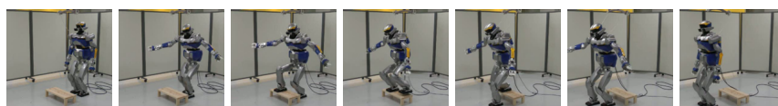
FIG 12. The HRP-2 over crossing a fifteen-centimeter platform: the HRP-2 takes steps the platform with one foot and over-cross it with the other.
