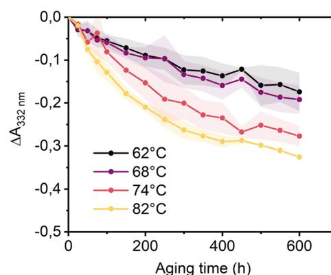
**Fig. 4 |** Changes in the absorbance at 332 nm of TPO1 films during UV aging with 305 nm LEDs at various temperatures (62, 68, 74, and 82 °C). The colored bands indicate measurement uncertainties.
