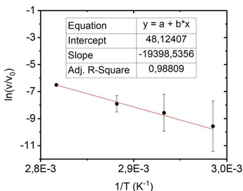
**Fig. 3 |** Determination of  $E_a$  for TPO1 (films irradiated with 305 nm LEDs at 20 W.m<sup>-2</sup>) using the Arrhenius method.
