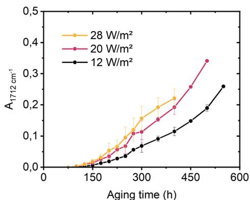
**Fig. 10** | Absorbance at  $1712\text{ cm}^{-1}$  (carboxylic acids) during aging of TPO1 at  $82\text{ °C}$  and at different UV irradiances and at 12, 20, and  $28\text{ W}\cdot\text{m}^{-2}$  (305 nm LEDs).
