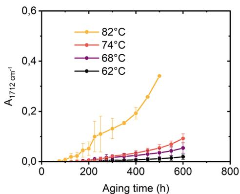
**Fig. 2 |** Absorbance at 1712 cm<sup>-1</sup> (related to carboxylic acids) during TPO1 film photoaging under 305 nm LEDs at various temperatures (62, 68, 74, and 82 °C).
