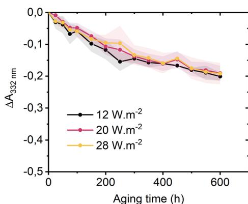
**Fig. 8** | Variation in the absorbance at 332 nm of TPO1 during UV aging under 305 nm LEDs at  $82^\circ\text{C}$  and varying levels of irradiance (12, 20, and  $28\text{ W}\cdot\text{m}^{-2}$ ). The colored bands indicate the measurement uncertainties.
