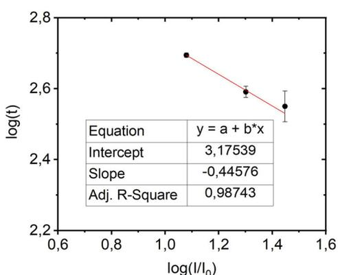
**Fig. 11** | Determination of the Schwarzschild factor for TPO1 films irradiated with 305 nm LEDs at  $82\text{ °C}$ .
