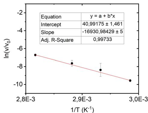
**Fig. 7 | Determination of Ea for TPO2 (films irradiated under 305 nm LEDs at 20 W.m<sup>-2</sup>) using the Arrhenius method.**
