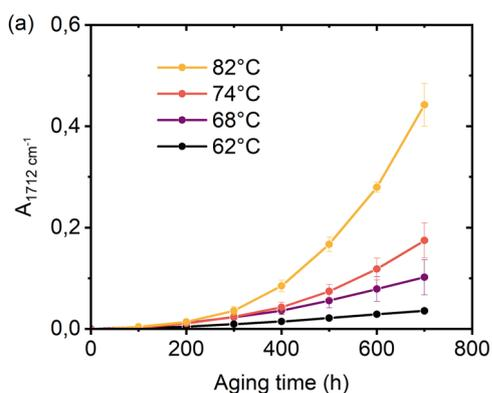
**Fig. 6 | Absorbance at 1712 cm<sup>-1</sup> (related to carboxylic acids) during TPO2 film photoaging under 305 nm LEDs at various temperatures (62, 68, 74, and 82 °C).**
