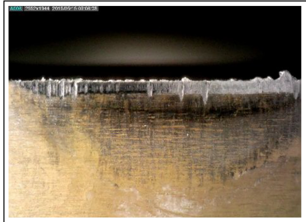
Figure 11. Tool flank wear: VB=0.294 mm, V_c=52.5 m/min, a_p=5.5 mm and t=18.83 min.
