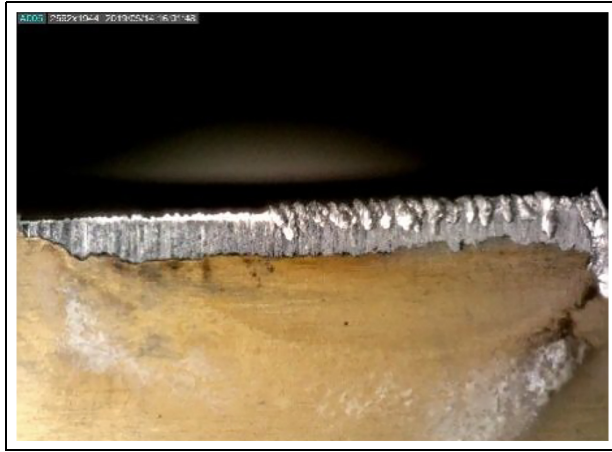
Figure 7. Tool flank wear: VB=0.091 mm, V_c=35 m/min, a_p=0.5 mm and t=4.99 min.
