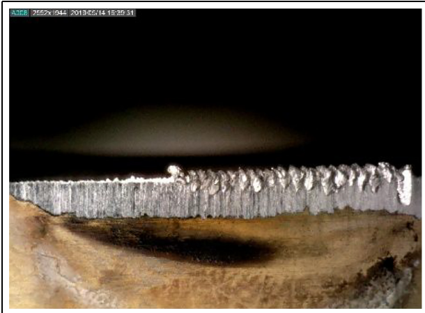
Figure 8. Tool flank wear: VB=0.123 mm, V_c=35 m/min, a_p=0.5 mm and t=10 min.
