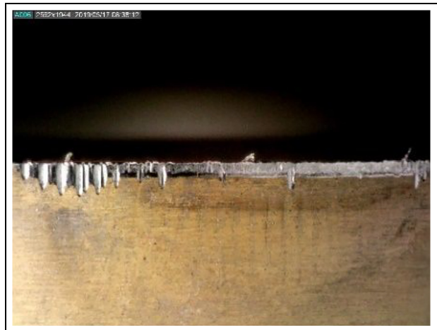
Figure 13. Tool flank wear: VB=0.066 mm, V_c=70 m/min, a_p=0.5 mm and t=2.26 min.
