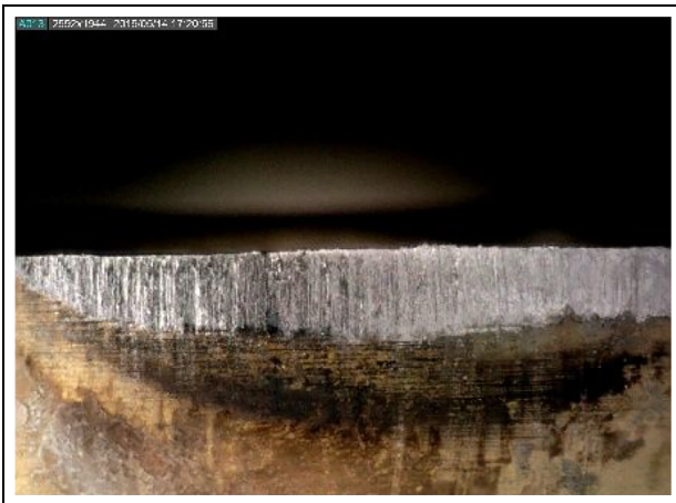
Figure 9. Tool flank wear: VB=0.292 mm, V_c=35 m/min, a_p=0.5 mm and t=54 min.
