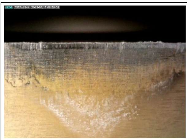
Figure 10. Tool flank wear: VB=0.071 mm, V_c=52.5 m/min, a_p=0.5 mm and t=3.01 min.
