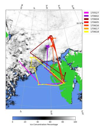
**Figure 1.** Flight paths for the ACLOUD flights with *Polar 6* aircraft included in the analysis overlaid on pack ice extend as of 2 June. Pack ice data are derived from measurements of the Advanced Microwave Scanning Radiometer 2 (AMSR2) at 89 GHz (http://www.seaice.uni-bremen.de, last access: 9 November 2022; Spreen et al., 2008).
