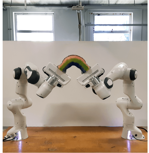
Fig. 1. Our experimental setup with two Franka Emika robots manipulating a foam octagonal cylinder. An overhead 3D camera provides the input for our approach.
