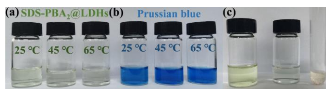
Fig. 6 The digital photos of (a) SDS-PBA 2 @LDHs and (b) pristine PB in the aqueous solution at 25°C, 45°C, 65°C and (c) pH=10 at 25°C, supernatant of SDS-PBA 2 @LDHs, supernatant of PB, and solution of PB (from left to right).
