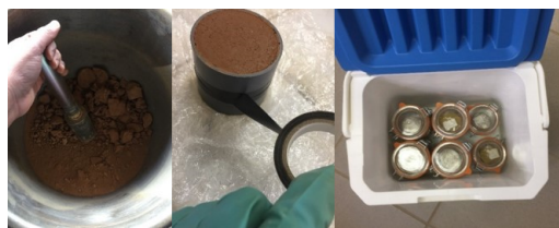
Figure 4: Test procedure to determine water retention curves.
