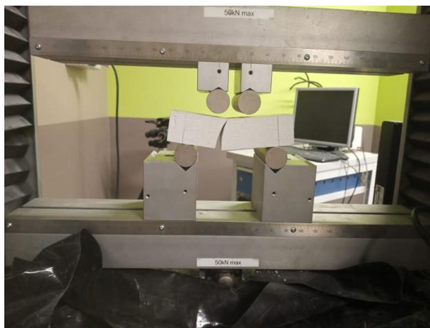
**Figure 4.** Flexural test setup.
