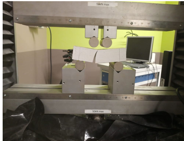
Figure 4. Flexural test setup.
