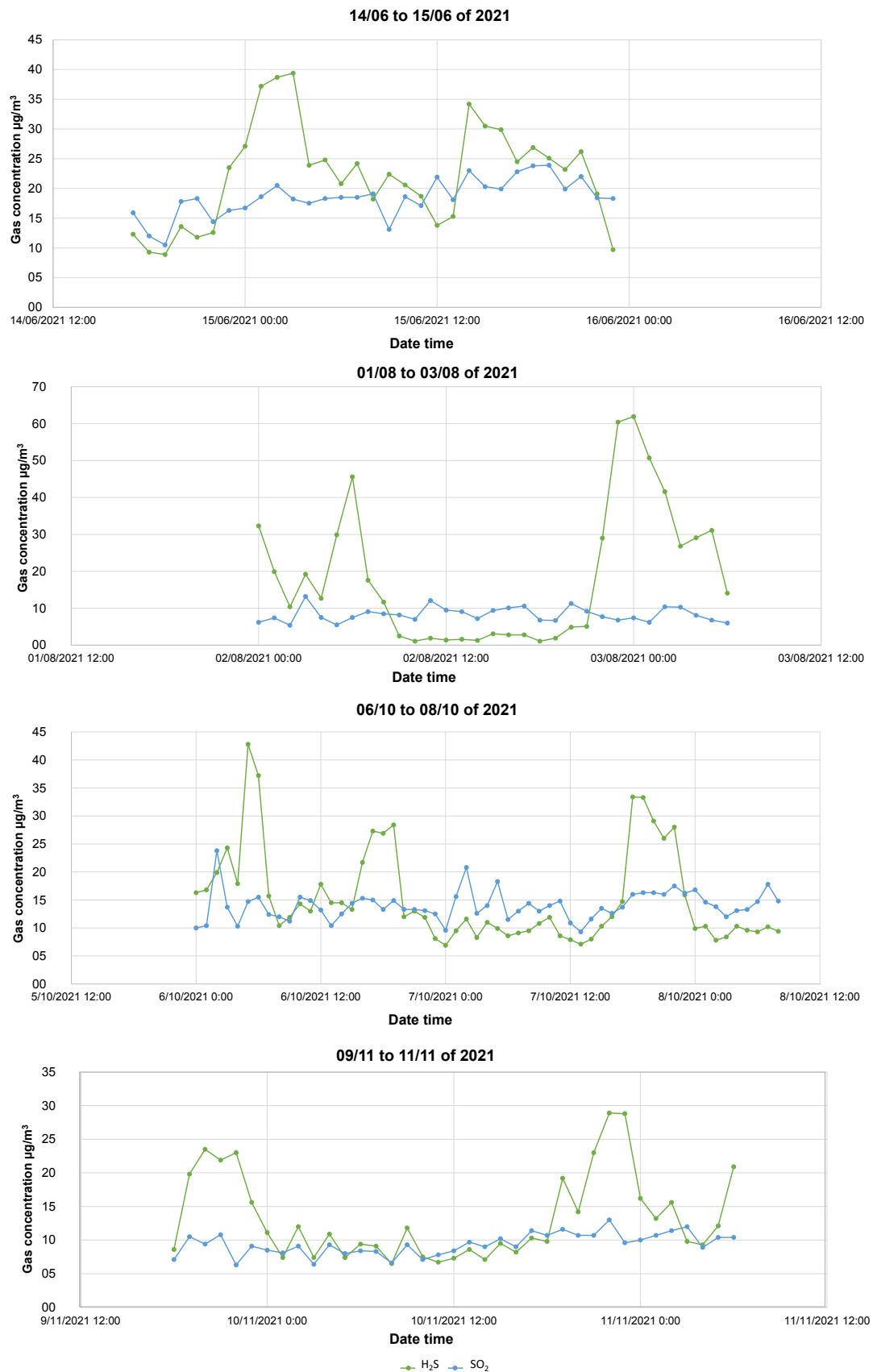
Figure 7: H 2 S and SO 2 behaviour per hours in the specific coincident dates from surveys and Gwad’Air reports. These data include background values for both gas species.
