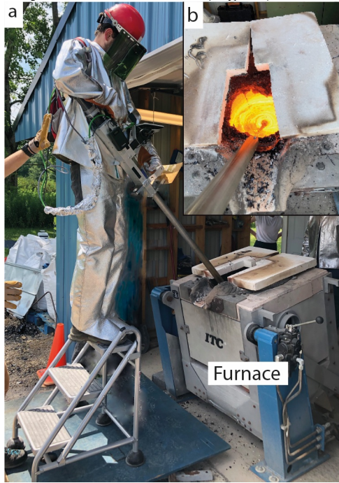
FIG 6: Measurements in a large-scale furnace. a) general view; b) view from the operator angle.
