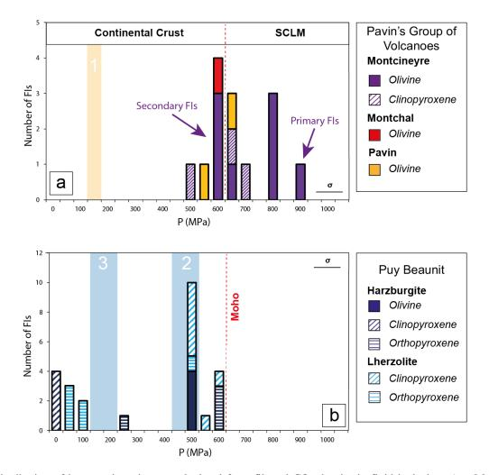
**Fig. 8.** Distribution of barometric estimates calculated from filtered  $CO_2$  density in fluid inclusions (see Methods) in crystals from (a) tephras of the Pavin's Group of Volcanoes and (b) mantle enclaves at Puy Beaunit. Shaded bar 1 highlights the pre-eruptive barometric conditions for the Pavin explosive event (Rondet et al., 2019). Shaded bars 2 and 3 are the two barometric modes identified from fluid inclusions in phenocrysts from lavas at Puy Beaunit (Bilal and Touret, 1977).
