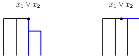
Figure 9 The two remaining possibilities for the clause gadget. The length 0 segments at each corner of the k -polygons are not represented. The black dots represent the length 0 segments we add for clauses with 2 literals.
