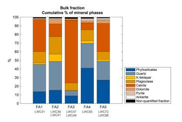
Fig. 2. Bulk mineralogical composition of the 8 LWC samples classified as a function of their facies.
