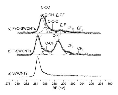
**Figure 1.** C<sub>1s</sub> XPS spectra, after background subtraction, of the a) pristine SWCNTs, b) SWCNTs fluorinated for 2h at 300°C, and c) final oxyfluorinated material.
