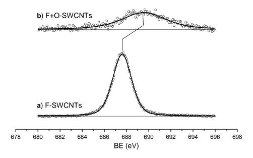
**Figure 2.** F<sub>1s</sub> XPS spectra, after background subtraction, of the a) SWCNTs fluorinated for 2h at 300 °C, and b) final oxyfluorinated material.
