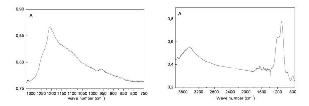
**Figure 3.** FTIR spectrum of the precursor fluorotubes (left) and final oxyfluoro-compound obtained (right).
