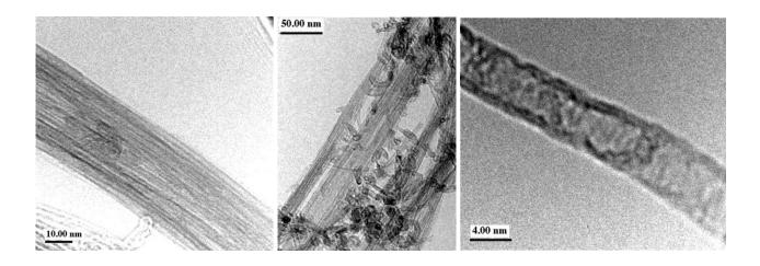
**Figure 4.** From left to right: TEM micrographs obtained from the pristine (bundle), fluorinated (bundle), and oxyfluorinated (individual tube) SWCNT samples, respectively.
