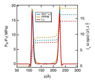
Figure 2: Profiles of  $p_{\rm N}(z) - p_{\rm T}(z)$  (left axis) and of its integral defined by  $\frac{1}{2}\gamma(z)$  (right axis) for the liquid-vapor of methane at T= 100 K for both spherically truncated and spherically truncated and shifted LJ potential models and for the dispersion term modeled by the PPPM method.
