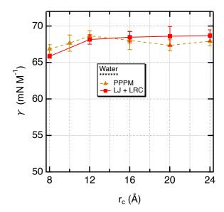
Figure 4: Surface tensions of water at  $T=300 \,\mathrm{K}$  calculated with different cutoffs  $(r_c)$ . The dispersion term is calculated using the PPPM method and a standard truncated LJ potential. Water was modeled using the TIP4P/2005 model.<sup>87</sup>
