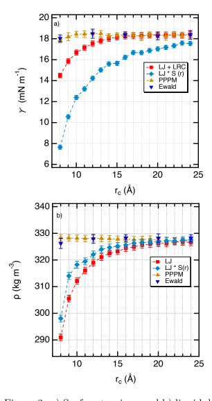
Figure 3: a) Surface tensions and b) liquid densities of the liquid-vapor equilibrium of methane at  $T=100\,\mathrm{K}$  calculated at different cutoffs  $(r_c)$  with several approaches for the dispersion term as indicated in the legend
