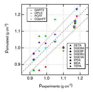
Figure 5: Correlation between experimental and calculated densities at  $T=300\,\mathrm{K}$ . The densities are calculated with different force fields and for various prepolymers and hardeners as indicated in the legend. The dotted lines represent simulated densities that deviate by  $\pm~5\%$  from experiments. The error bars are less than symbols' size.
