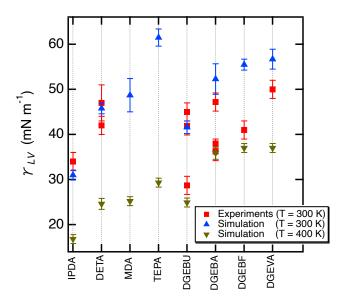
Figure 6: Surface tensions of the liquid-vapor equilibrium of pure polymers and hardeners calculated with the PCFF model. The experimental surface tensions are only available at 300 K. These values are either taken from the literature, from our own experiments or deduced from  $-\frac{d\gamma}{dT}$ . The origin of these data is specified in Table 1. The simulated surface tensions at 400 K are given for completeness.
