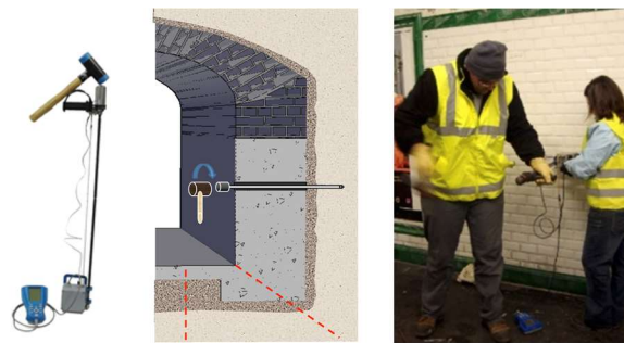
Figure 2. Principle and example of penetrometric and geodendoscopic measurements
