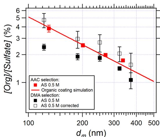
**Figure 5.** Influence of instrumental conditions and instrument inter-comparison: AAC selection (red squares, EXP P1), DMA selection (black squares, EXP P6), and multi-charging correction (white squares). The red line represents the calculation simulating organic coated compounds at the AS particle surface using Eq. (3) with a surface density of  $1.1 \times 10^{-3} \text{ g m}^{-2}$  (selected from Fig. 4).
