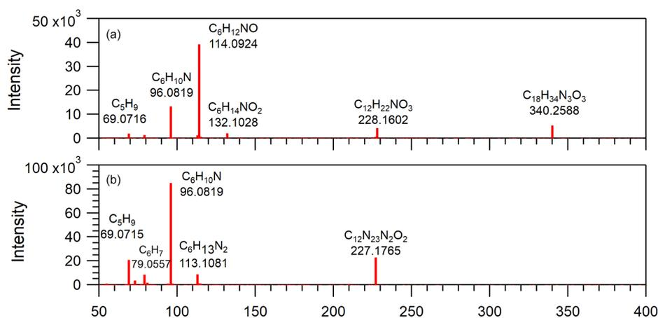
**Figure 8.** Mass spectra obtained from LC/ESI<sup>+</sup>-MS/MS measurements of two detected compounds in EXP C9. The [M+H]<sup>+</sup> ions were detected at (a)  $m/z$  340, using a collision energy of 25 eV, and (b)  $m/z$  227, using a collision energy of 20 eV.
