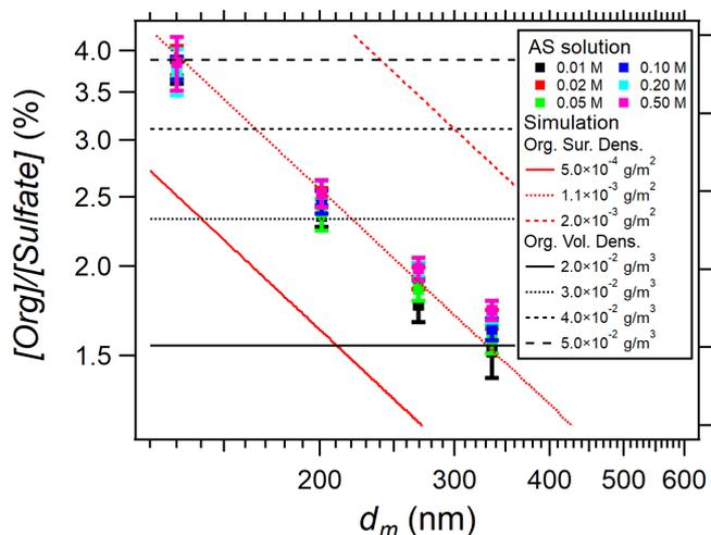
**Figure 4.**  $[\text{Org}]/[\text{Sulfate}]$  in AS aerosols versus particle mobility size ( $d_m$ ) during EXP P1 scanning the six nebulized AS concentrations (0.01–0.5 M). The colored dots (with error bars) are the experimental data, while the red and black lines represent the calculated  $[\text{Org}]/[\text{Sulfate}]$  considering either surface coating of organic matter (in red from Eq. 3) or internal mixing (in black from Eq. 4).
