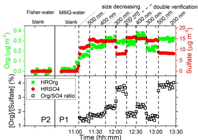
**Figure 2.** Mass concentrations of total organic matter, sulfate, and  $[\text{Org}] / [\text{Sulfate}]$  ratio as a function of time during one cycle performed in EXP P1 at an AS concentration of 0.01 M. Background signal obtained with pure water in EXP P1 and P2 is also shown for quality check and for comparison between the two types of water with different purity.
