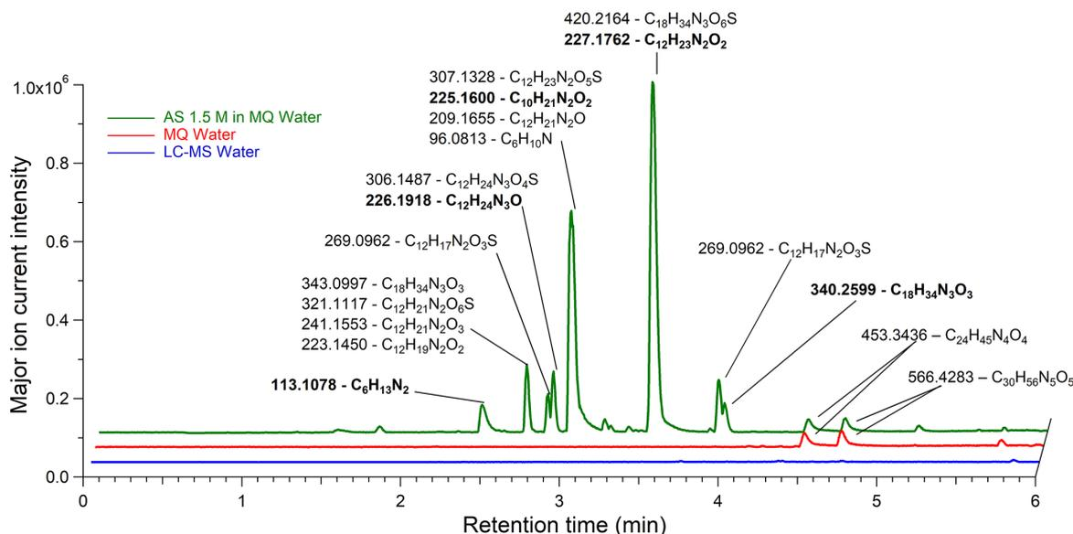
**Figure 7.** LC/ESI<sup>+</sup>-MS base peak chromatogram of Milli-Q water, Fisher water, and AS (99.5 %) solution of 1.5 M (EXP C1) with corresponding major ion masses associated with raw formulas. The bold ion masses and proposed raw formula were studied in MS-MS (EXP C9). Ions displayed in boldface were detected in their [M - H]<sup>-</sup> form in LC/ESI<sup>-</sup>-MS (in EXP C6-C8).
