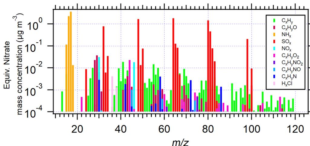
**Figure 3.** Unit-mass resolution spectra (averaged over 12 measurements, converted from the high-resolution data) of AS aerosol particles ( $d_a = 200$  nm) in EXP P1, performed at an AS concentration of 0.5 M.
