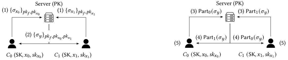
(a) Computation of y = f(x_0, x_1) where the function f is simulated by the server using PK over \sigma_{x_0} and \sigma_{x_1} the encoding of respectively the input x_0 and x_1 .
