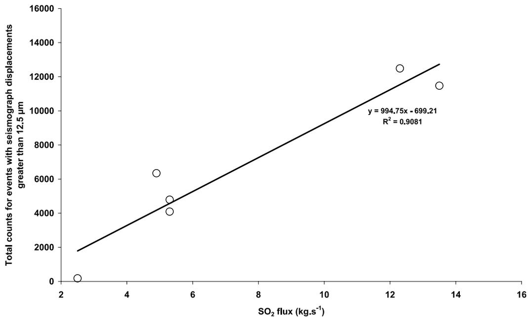
**Figure 4.** Correlation plot between seismic events and SO<sub>2</sub> emission rates. Emissions rate which correspond to P5 and P7 were omitted because of high gas discharge which occurred with no significant seismic events and lack of seismic data respectively.
