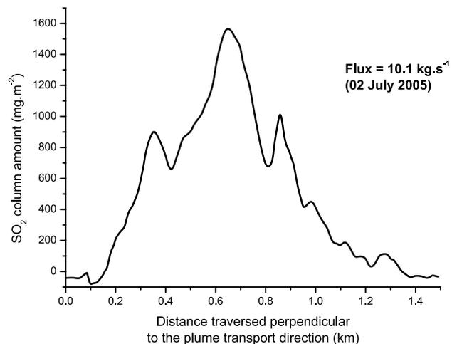
**Figure 2.** Representative plot of a cross sectional profile of SO<sub>2</sub> concentration for one traverse obtained under the Yasur plume in July 2005. The three peaks correspond to individual plumes emitted from the three active vents in the crater.
