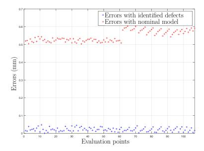
Figure 10: Norm of the error between measured and simulated position of the end effector of the Tripteor X7
