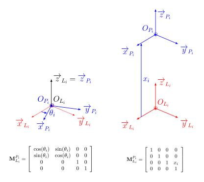
Figure 2: Definition of the necessary frames and matrices for the rotation and the translation movement
