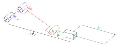
Kinematic model of slider-rod-crank mechanism
