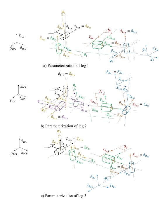
Figure 5: Parameterization of the Tripteor X7 legs
