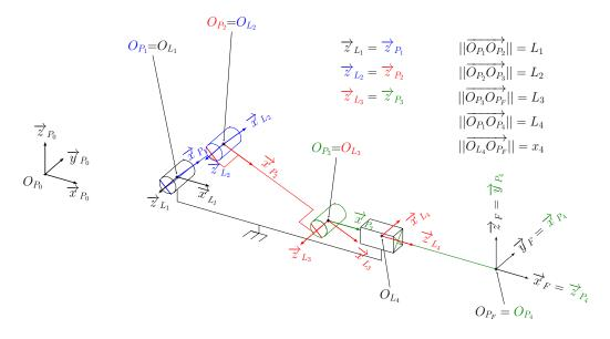
Figure 3: Parameterization of the slider-rod-crank mechanism
