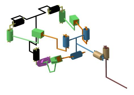
Figure 4: Kinematic model of the Tripteor X7, the black part corresponds to the fixed platform, the cyan part to the mobile platform and the dark brown hosts the spindle of the machine-tool
