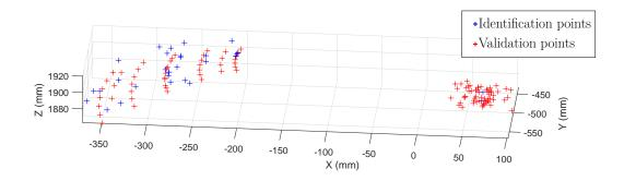
Figure 8: Measured points in the Tripteor X7 workspace. Red dots are identification points, blue dots are validation points
