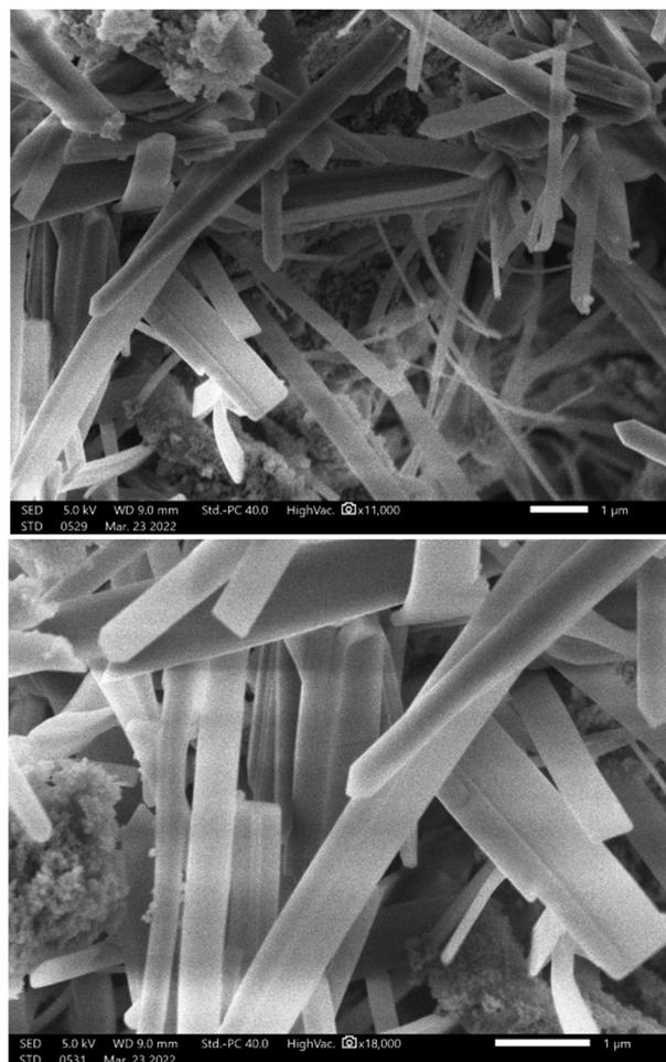
Fig. 8 SEM images of Mn-LDH obtained for  $x = 0.25$ .
