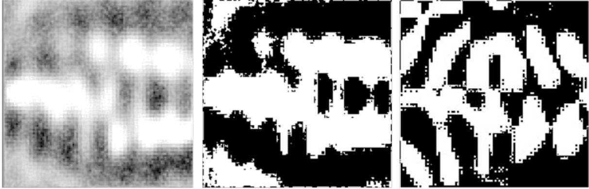
Figure 3: The demultiplexer in the highest resolution ( $202 \times 202$ ) and for the lowest value of the cost function: after BFGS (left), after BFGS and discretization (middle) and after having run the algorithm Lengler equipped with the smoothing operator (right). The material with high permittivity is in black, while air is represented in white. There are significant differences before the discrete algorithm begins and the final result.
