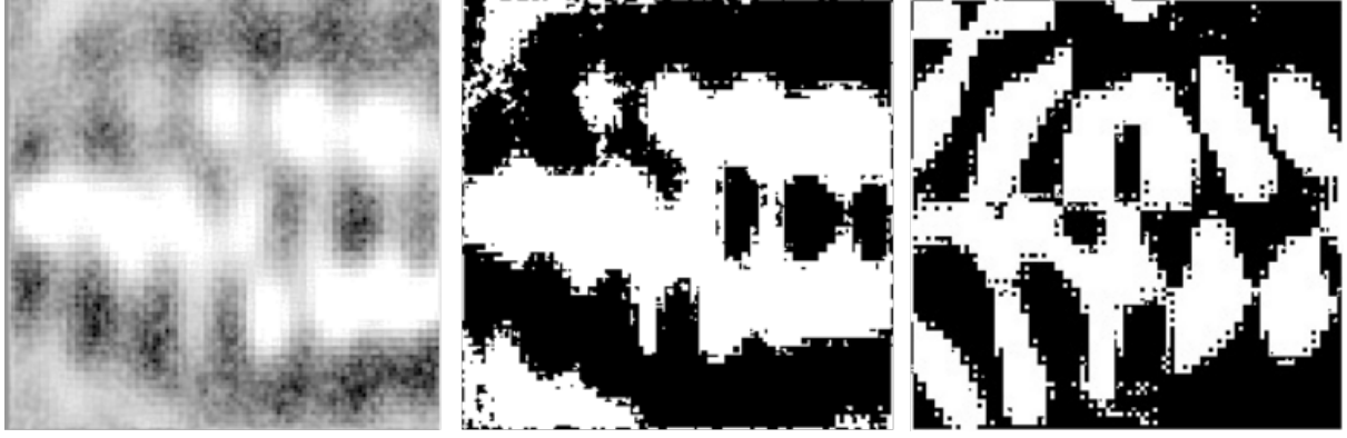
Figure 3: The demultiplexer in the highest resolution ( 202 \times 202 ) and for the lowest value of the cost function: after BFGS (left), after BFGS and discretization (middle) and after having run the algorithm Lengler equipped with the smoothing operator (right). The material with high permittivity is in black, while air is represented in white. There are significant differences before the discrete algorithm begins and the final result.
