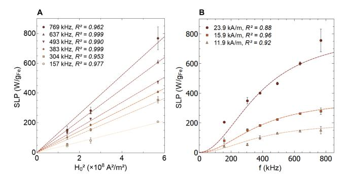
Figure 11. Evolution of measured specific loss power with the square of AMF amplitude (A) and with field frequency (B) along with the fit with LRT model. Adjusted R<sup>2</sup> values are indicated for goodness of fit
