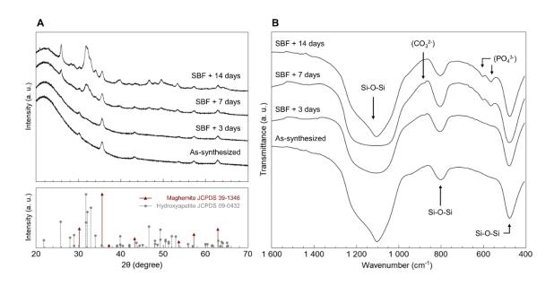
Figure 7. XRD patterns (A) and FTIR spectra normalized to the Si-O-Si band at 475 cm-1 (B) of heterostructured NPs before and after up to 14 days of immersion in SBF
