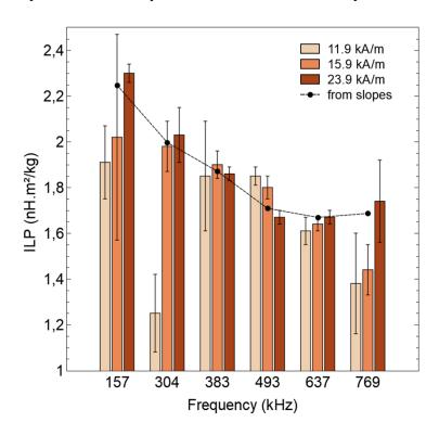
Figure 12. Evolution of intrinsic loss power (ILP) with field frequency. Black circles: values obtained from the fits of the SLP versus  $H_0^2$  curves (the dashed line is a guide to the eye). Vertical bars: values calculated for each set of AMF parameters, from the equation ILP =  $SLP/f \cdot H_0^2$
