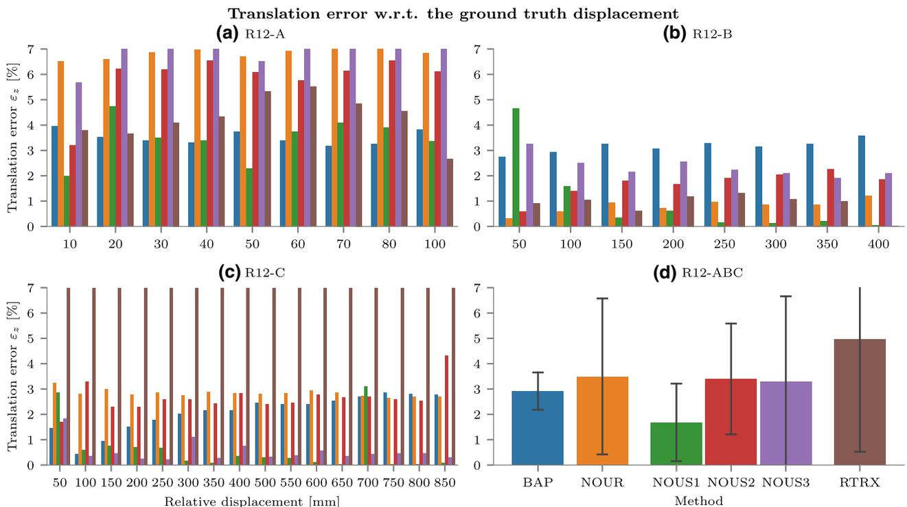
**Fig. 8** Translation error along the  $z$ -axis with respect to the ground truth displacement from the closest frame, for datasets R12-A (a), R12-B (b) and R12-C (c). The error  $\epsilon_z$  is expressed in percentage of the estimated distances, and truncated to 7% to ease the readability and the comparison. The mean error with its confidence interval across all datasets for
