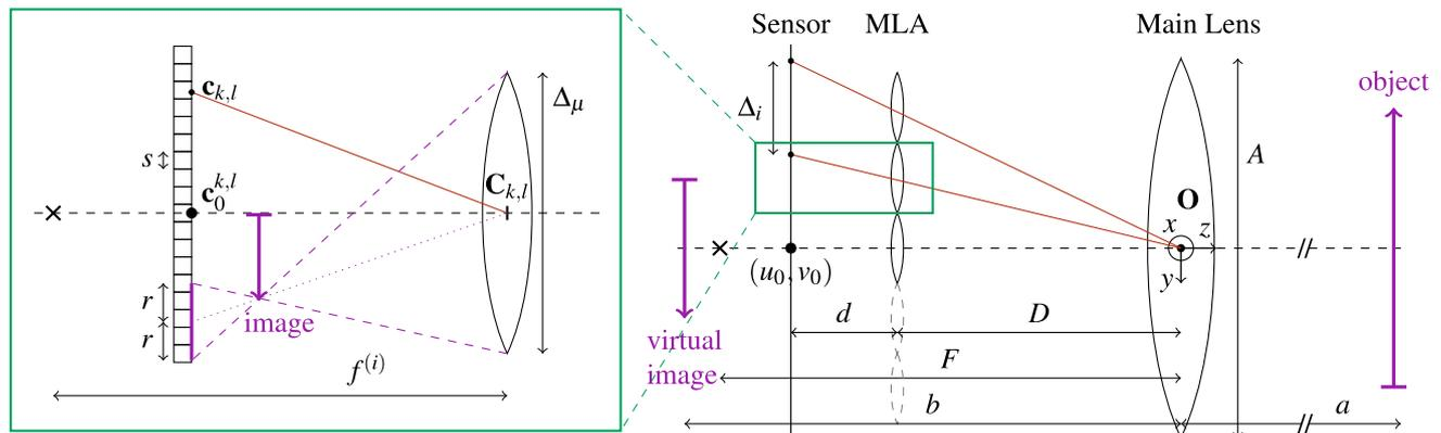
**Fig. 3** Focused plenoptic camera model in Galilean configuration with the notations used in this paper. Object points are projected by the main lens behind the MLA into a virtual intermediate space, and then re-imaged by each micro-lens onto the sensor.
