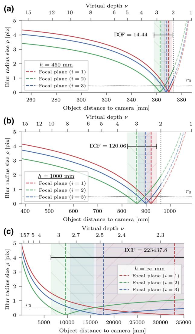
**Fig. 10** Blur profile, including each micro-lens type, in object space, at different focus distances: **a**  $h = 450$  mm; **b**  $h = 1000$  mm; and **c**  $h = \infty$  mm. Focal planes and depth of fields are illustrated for each type. The blur radius is expressed in pixel as function of the object distance to the camera in mm. Corresponding virtual depth is reported on the secondary  $x$ -axis.
