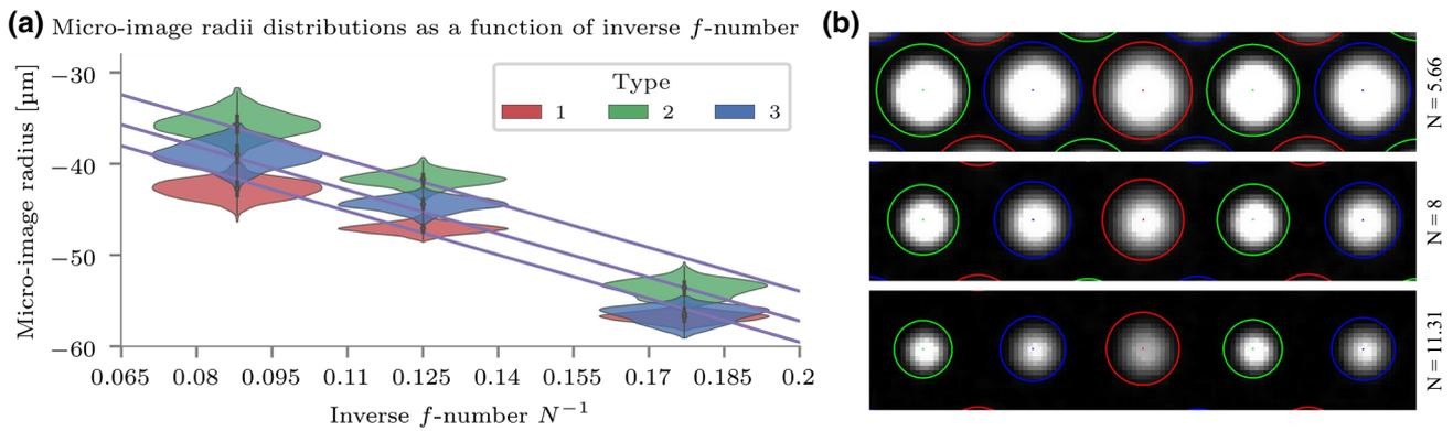
**Fig. 5** **a** Micro-image radii as function of the inverse  $f$ -number (in magenta), with their distributions represented by the violin-boxes, for our camera consisting of  $I = 3$  different types. **b** Each type of micro-
