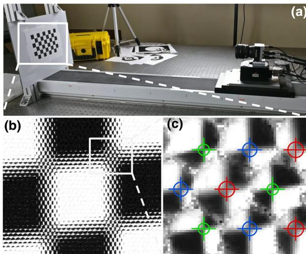
**Fig. 1** The Raytrix R12 multi-focus plenoptic camera used in our experimental setup (a), along with a raw image of a checkerboard calibration target (b). The image is composed of several micro-images with different amounts of blur, arranged in a hexagonal grid. In each micro-image, our Blur Aware Plenoptic (BAP) feature is illustrated by its center and its blur circle (c).
