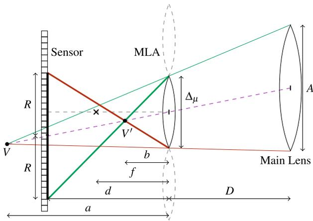
**Fig. 4** Formation of a micro-image with its radius  $R$  through a micro-lens while taking a white image using a light diffuser, at an aperture  $A$ , in Keplerian internal configuration. The point  $V$  is the vertex of the cone passing by the main lens and the considered micro-lens.  $V'$  is the image of  $V$  by the micro-lens and  $R$  is the radius of its blur circle.
