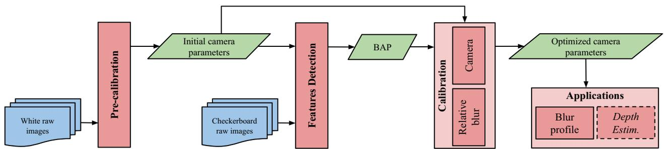
**Fig. 2** Overview of our proposed method: first, the pre-calibration step retrieves initial camera parameters from white raw images at different apertures; then followed by the detection of BAP features that are used by the camera calibration process and calibration of the relative blur;
