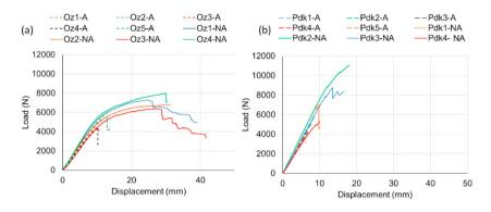
Fig 4:Load displacement curves of single lamella, (a) Oz-A Vs Oz-NA, (b) Pdk-A Vs Pdk-NA.
