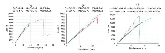
Fig 5:Load displacement curves of combined GLT beam, (a) Oz-Pdk-A1 Vs Oz-Pdk-A2, (b) Pdk-Oz-A1 Vs Pdk-Oz-A2, (c) Pdk-Oz-Pdk-A Vs Oz-Pdk-Oz-A
