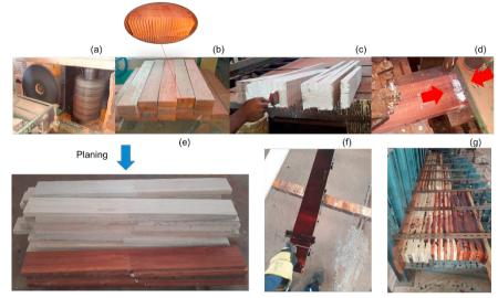
Fig 1: Gluing process, (a) Cutterheads ; (b) Finger jointed lamella; (c) Coating finger joints with Prefere adhesive; (d) Pressurize (2 s); (e) Lamellas with finger joint and planed, (e) Coating with PRF adhesive (g) Pressurize (24h);
