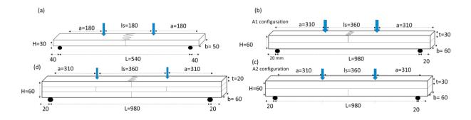
Fig 2: Mechanical principle of the 4-point bending test, (a) Single lamella with finger joint, (b) DUO in A1 configuration, (c) DUO in A2 configuration, (d) TRIO
