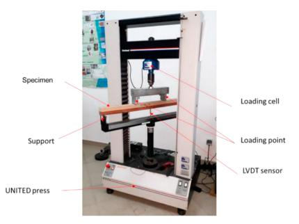
Fig 3: Experimental device
