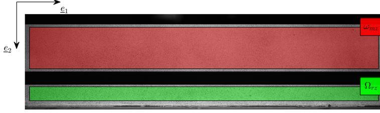
Figure 2: Reference image, which defines the reference state. Two regions of interest are defined here.  $\omega_{mz}$  is defined on the workpiece surface and corresponds to the measurement zone. A speckle has been painted on this surface.  $\Omega_{rz}$  is the workpiece support surface, a speckle has also been painted on it.
