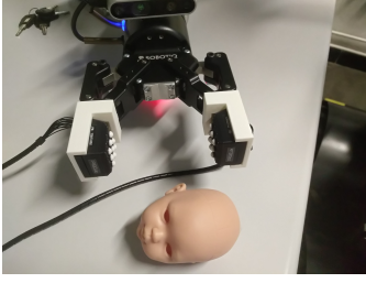
Fig. 6. Integrated tactile sensors.
