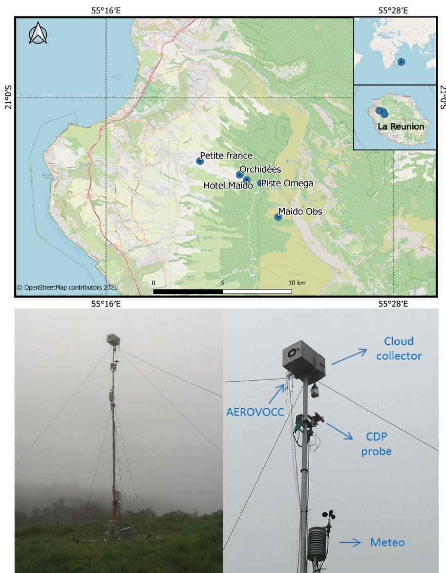
**Figure 1.** Locations of Piste Omega and other instrumented sampling sites in Réunion. Photo of the mast (10 m height) deployed during the BIO-MAÏDO project integrating the cloud water collector, cloud droplet probe (“CDP”), meteorological station (“Meteo”), and gas-phase collection (“AEROVOCC”).
