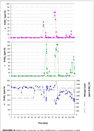
**FIGURE 9** | Nitrogen species at the nitrification compartment outlet during the integration experiments where Compartment 3 and 4a are connected in the liquid phase and Compartment 4a and 5 in the gas phase. [**Dotted pink:** N-NH<sub>4</sub><sup>+</sup> (ppm); **Square green:** N-NO<sub>2</sub><sup>-</sup> (ppm); **Triangle blue:** N-NO<sub>3</sub><sup>-</sup> (ppm)].
