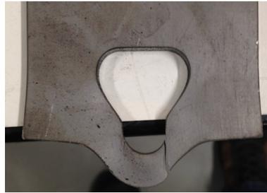
(c) Failure by shear and bearing
