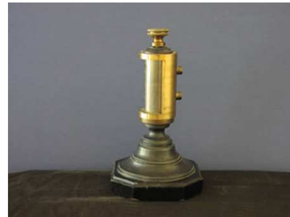
Figure 1: Revolute or Pin Kinematic Pair.
