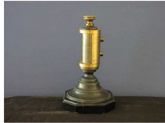
Figure 1: Revolute or Pin Kinematic Pair.
