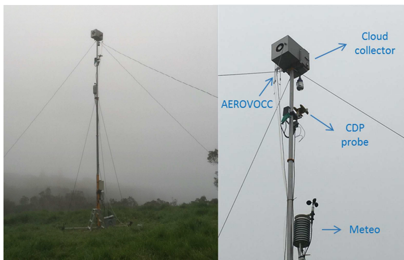
280 Figure 1. Location of Piste Omega and other instrumented sampling sites at Reunion Island. Photo of the mast (10 m height) deployed during the BIO-MAÏDO project integrating the cloud water collector, cloud droplet probe (“CDP probe”), meteorological station (“Meteo”) and gas phase collection (“AEROVOCC”). © OpenStreetMap contributors 2021. Distributed under the Open Data Commons Open Database License (ODbL) v1.0.
