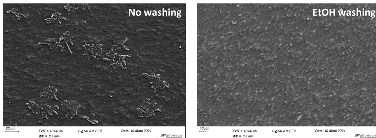
Figure 6: SEM images ( \times 400 ) of unwashed (left) and EtOH-washed (right) PE-770-1 films.
