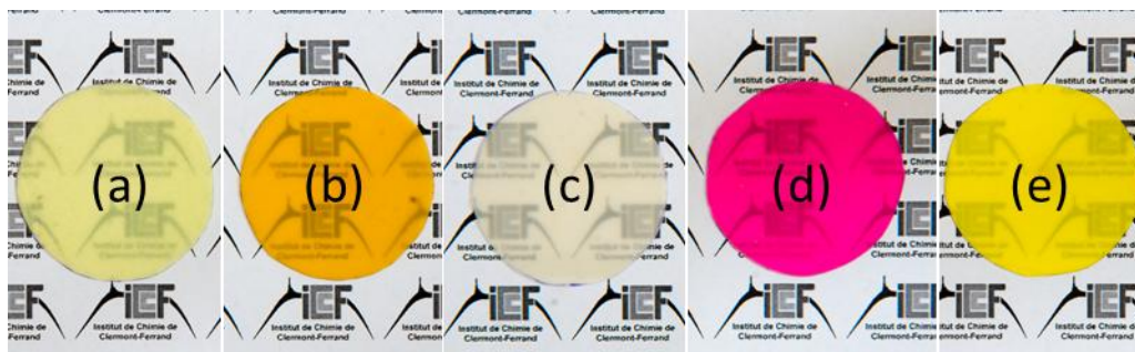
Fig. 7. Pictures under daylight of the different silicone/LDH-PAO (40 wt%) films: (a) LDH-AO/C343, (b) LDH-AO/HPTS, (c) LDH-AO/C3C, (d) LDH-AO/RhB and (e) LDH-UV/HPTS.
