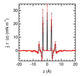
Figure A1. Profile of the surface tension  $(mN m^{-1})$  of the graphene monolayer water interface along the z-dimension. The statistical fluctuations are represented by error bars calculated over 5 block-averages during the acquisition phase.
