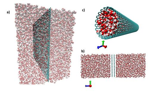
Figure 2. Typical configurations of a) a graphene monolayer layer, b) a graphene bilayer and c) a carbon nanotube (CNT) in interaction with water molecules at 300K where the z-direction is normal to the graphene surface for planar interfaces.
