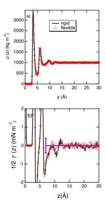
Figure 6. a) Water density and b) interfacial tensions profiles calculated with a static and flexible graphene sheet by using the RFD method and  $r_c = 12$  Å. The statistical fluctuations calculated as a function of z (see Figure A1) are shown at two typical z-positions, z = 7 and 24 Å in b).
