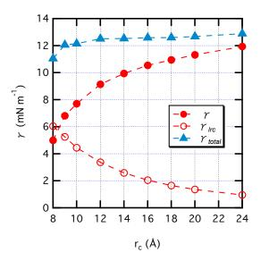
Figure 1. Liquid-vapour surface tensions of methane calculated at 125 K for different cutoff values. The long-range corrections ( $\gamma_{lrc}$ ) to the surface are calculated using the local Janeček approach[13, 15] and the short range part  $\gamma$  using the Irving-Kirkwood definition [16, 17]. The total surface tension  $\gamma_{total}$  sums then  $\gamma_{lrc}$  and  $\gamma$ .
