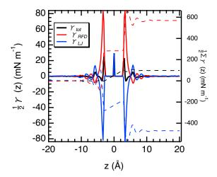
**Figure D1.** Local interfacial tensions of water molecules interacting with a graphene monolayer calculated with RFD and a cutoff radius of 12 Å. The profiles of the LJ and electrostatic parts are represented for comparison. The interfacial tensions are read on the right axis.
