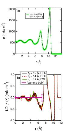
Figure 8. Profiles of the a) radial density of water molecules confined in the nanotube and b) interfacial tensions as a function of the radial distance r. The profiles are represented on half the boxlength. The statistical fluctuations calculated as a function of z (see Figure A1) are shown at two typical z-positions, z=0 and 7 Å in b).
