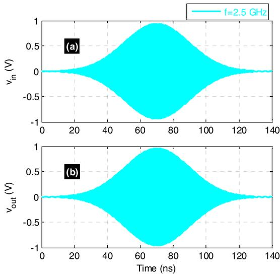
**FIGURE 12.** Time-domain simulation results of the lill-circuit touchstone S-parameter with Gaussian pulse input modulating  $f_c = 2.5$  GHz sine carrier.
