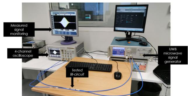
**FIGURE 13.** Photograph of the time-domain experimental setup with the NGD lill-circuit prototype.
