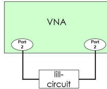
FIGURE 5. Illustrative diagram of the S-parameters experimental setup.
