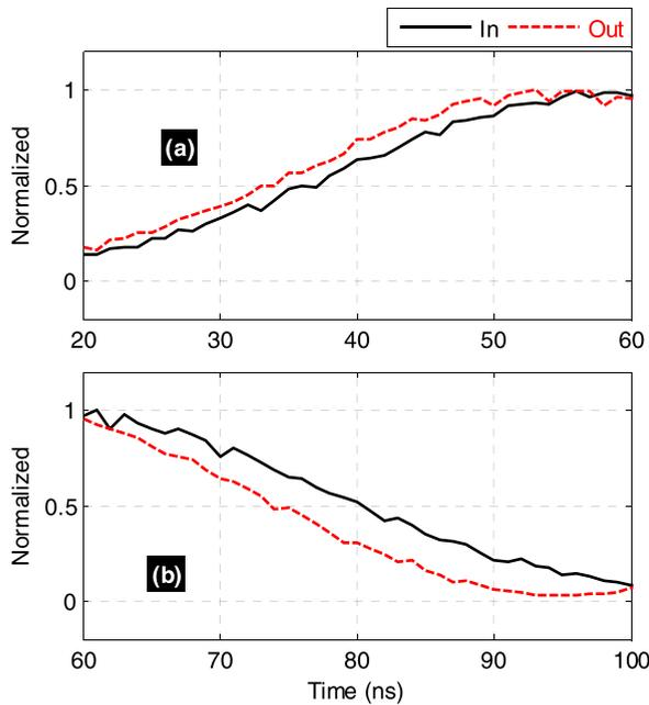
**FIGURE 17.** Zoom in of (a) leading and (b) tailing edges of measured input and output normalized transient signals shown in Fig. 16(b).
