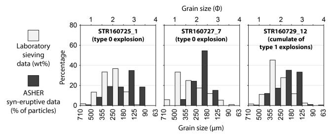
Figure 7 – Grain size of the three collected ash samples measured both by the ASH collector and sizER (ASHER) instrument and by laboratory sieving.
