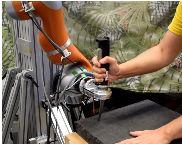
Figure 29. Foam cutting along the global y-direction.
