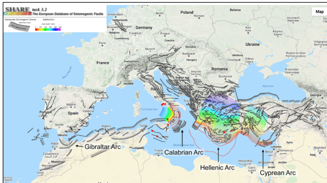
Figure 1.3: Distribution of seismogenic faults, composite seismogenic sources and active subduction zones (bold black line and gray zone represent fault top trace and fault dipping plane, respectively), modified from the European Database of Seismogenic faults (Basili et al., 2013). The active volcanoes mentioned in the text above are plotted as red squares.
