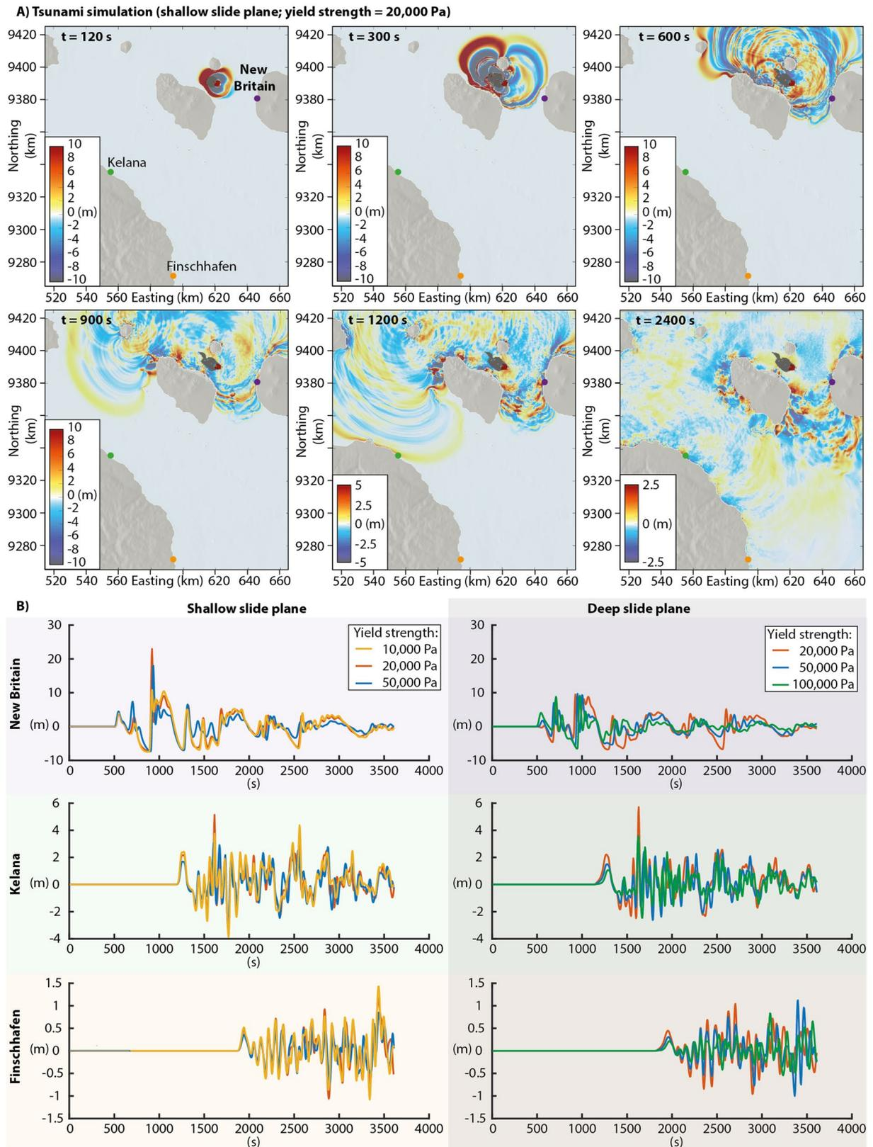
**Fig. 6** a Simulation of the propagation of the 1888 Ritter Island tsunami. b Virtual tide gauges at New Britain, Kelana and Finschhafen for simulations with various yield strength values for the shallow and the deep slide planes
