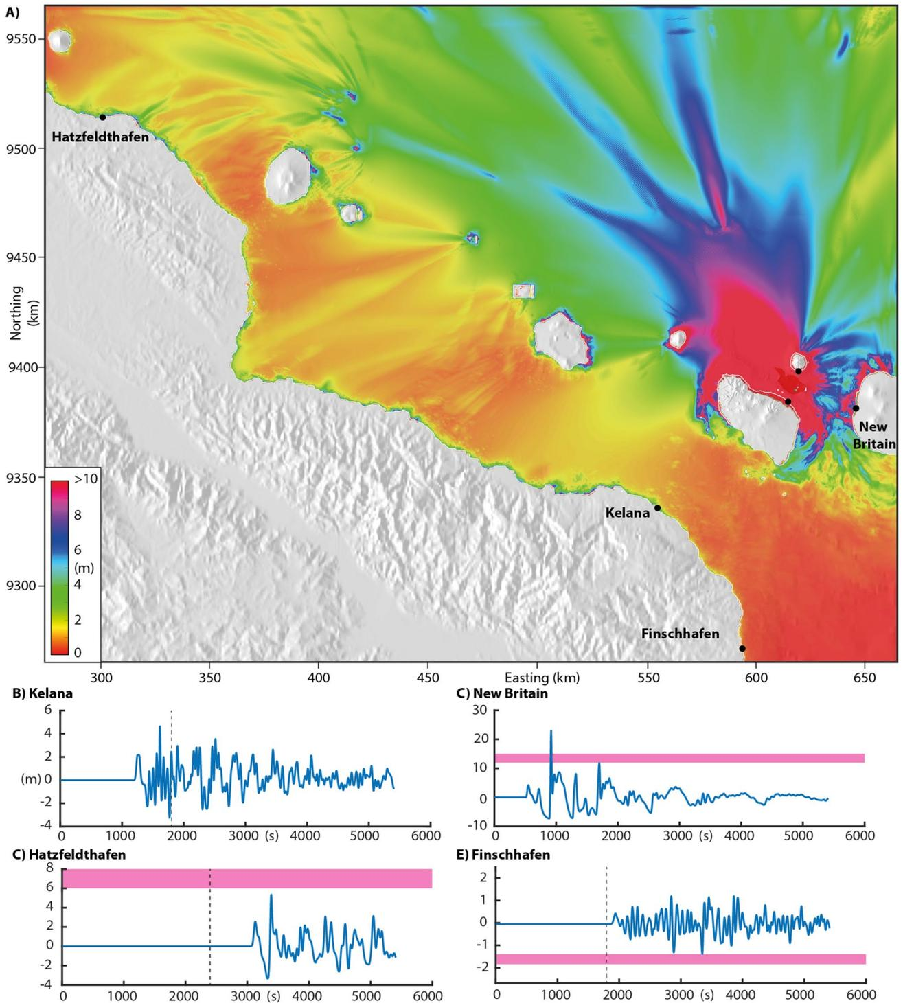
**Fig. 8** a Map showing the maximum tsunami height for simulation S19 of the 1888 Ritter Island tsunami. b–e Virtual tide gauges and the tsunami heights (pink squares) and arrival times (dashed lines) from historic eyewitness accounts
