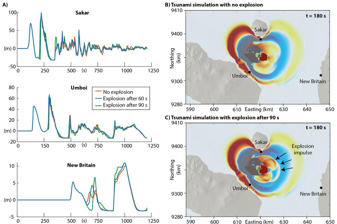
**Fig. 7** **a** Virtual tide gauges at Sakar, Umboi and New Britain for simulations with an explosive eruptions after 60 s and 90 s as well as without an explosion. **b** Propagation of the 1888 Ritter Island tsunami
