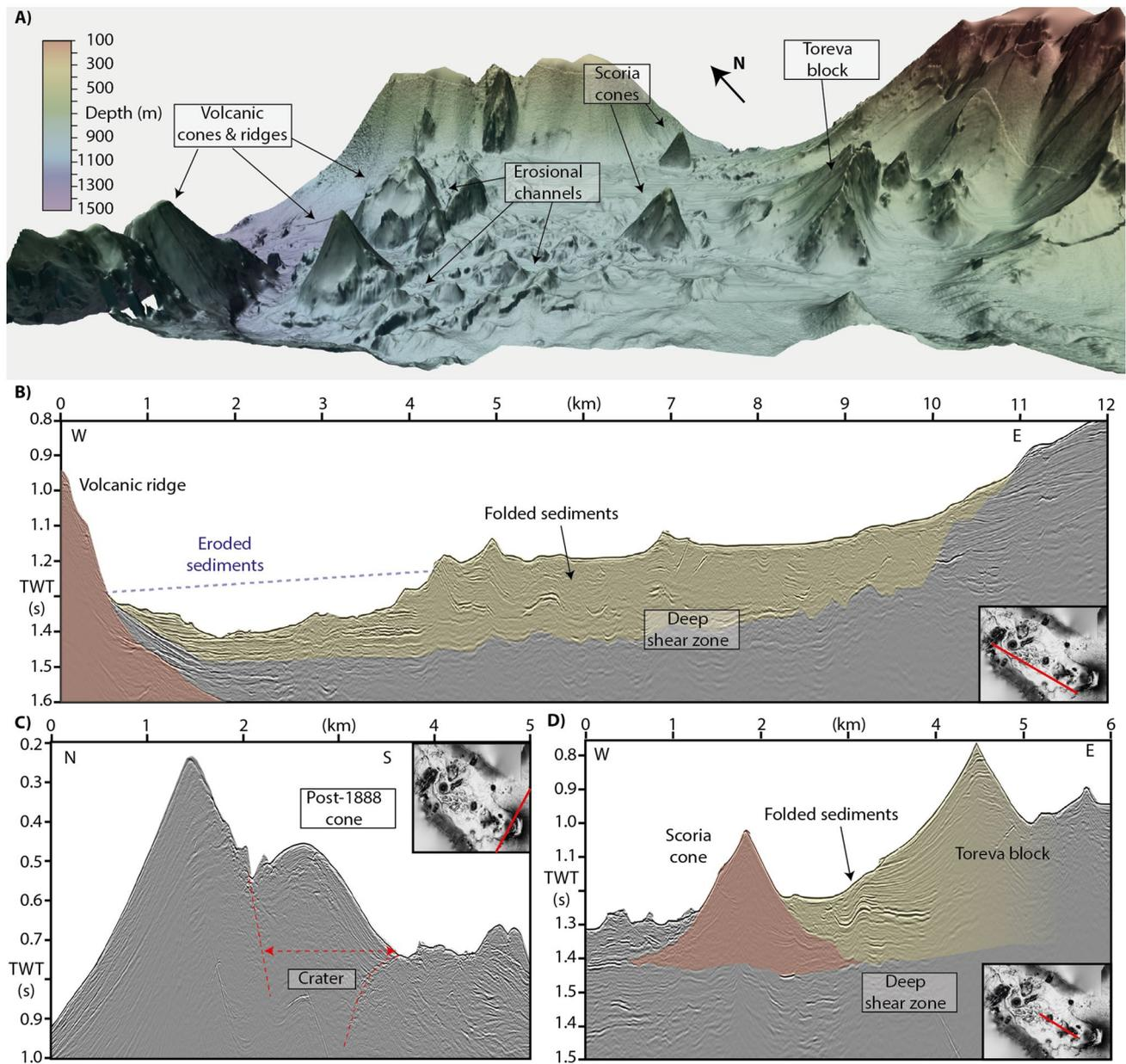
**Fig. 2** **a** 3D view on the proximal deposits of the 1888 Ritter Island sector collapse. **b** Seismic profile covering the failed edifice of Ritter Island, the deformed seafloor sediments (yellow), and the volcanic ridge (red) to the west. **c** Seismic profile through the failed volcanic
