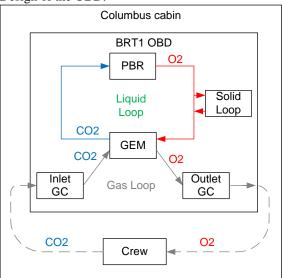
Figure 1.b (right) BRT1 On board demonstratorflow principle (GC means Gas Conditioning).
