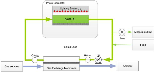
Figure 2. Piping & Instrumentation Diagram of the BBM
