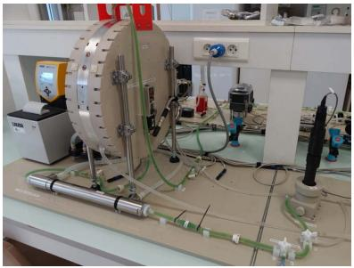
Figure 3. PBR during life test with visible cyanobacteria in LL.
