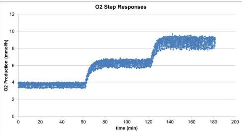
Figure 9. O<sub>2</sub> Production step responses (20 W/m<sup>2</sup>, 35 W/m<sup>2</sup> and 50 W/m<sup>2</sup>)
