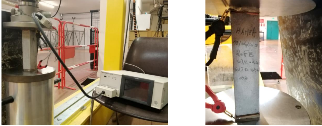
Fig. 3: Compression test setup
