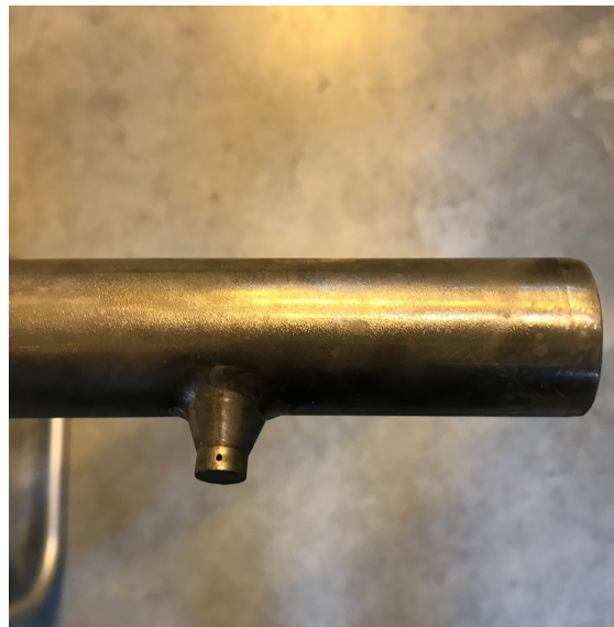
Figure 2: Detail of the measuring tip of the Pavlov tube.
