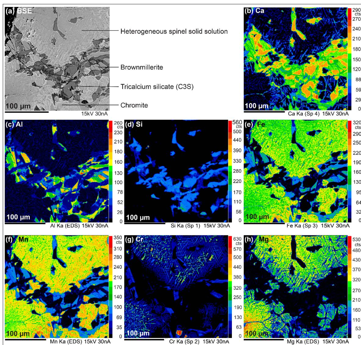
**Figure 5.** Chemical maps of a selected 1 mm grain from sample Mix 1 (Block 5 grain 07). (a) BSE (back-scattered electrons) image; (b–h) quantified chemical maps of Ca, Al, Si, Fe, Mn, Cr, and Mg obtained by EMPA.
