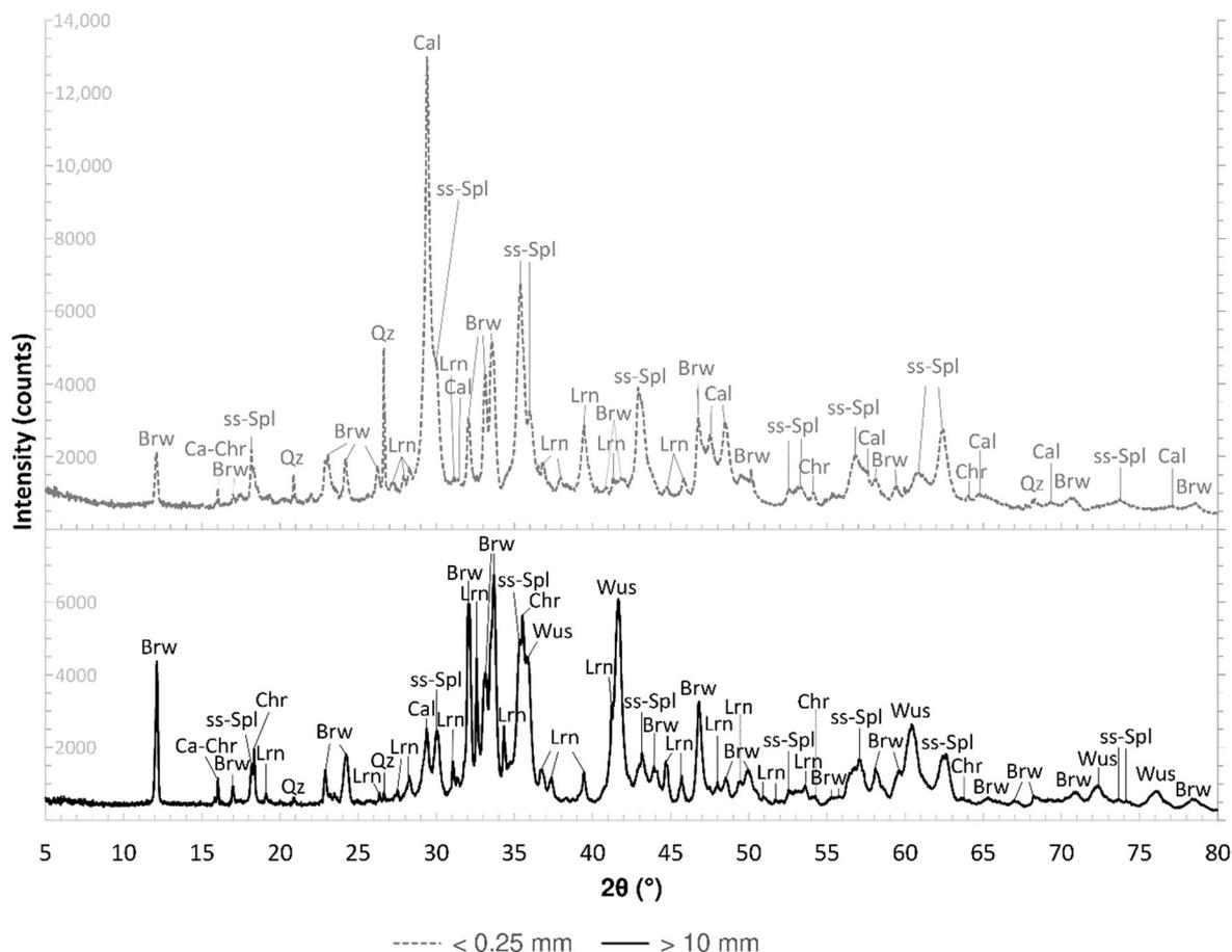
**Figure 2.** X-ray diffraction (XRD) pattern for the fractions <0.25 mm and >10 mm (Wus = wustite, ss-Spl = spinel solid solution, Chr = chromite, Brw = brownmillerite, Ca-Chr = calcium chromite, Lrn = larnite, Cal = calcite, Qz = quartz).
