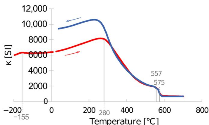
**Figure 7.** Variation of the magnetic susceptibility ( $\kappa$ ) during heating-cooling cycle (red and blue line respectively) from  $-192\text{ }^{\circ}\text{C}$  to room temperature and from room temperature to  $700\text{ }^{\circ}\text{C}$ .
