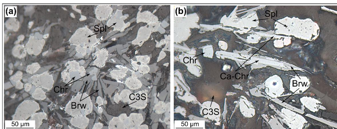
**Figure 3.** Reflected light microphotographs taken by optic microscope Leica DM4500 P on selected 1 mm grains from sample Mix 1 (a) Block 1–grain 25 (b) Block 5–grain 16. Abbreviations: spinel solid solution (Spl), chromite (Chr), brownmillerite (Brw), tricalcium silicate (C3S), calcium chromite (Ca-Chr).
