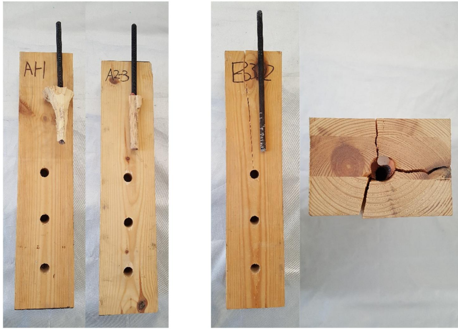
Fig. 6 Failure mode: timber-adhesive interface failure (left) and splitting failure (right)
