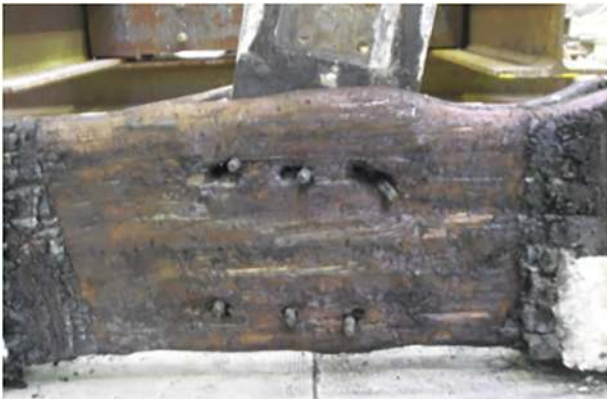
Fig. 7. Large plastic deformations observed after a fire test of steel-to-timber connection in bending (Fig. 3c).
