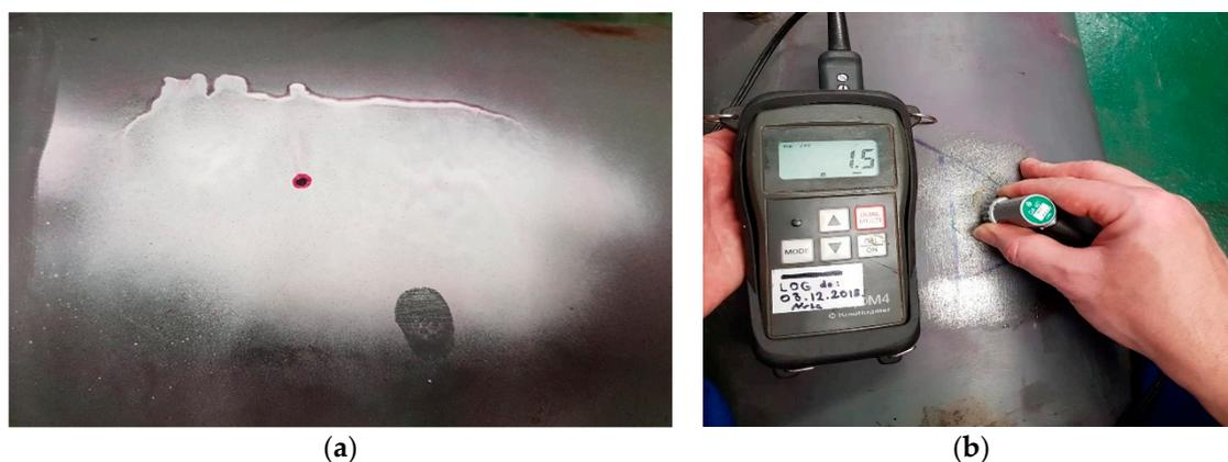
**Figure 2.** Example of non-destructive testing of rotating machinery equipment: (a) liquid penetrant testing, (b) ultrasonic thickness testing.
