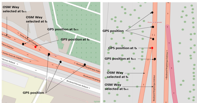
Fig. 9: Scenarios where the map matching algorithm selects the wrong OSM Way and leads to a false lanes number estimation
